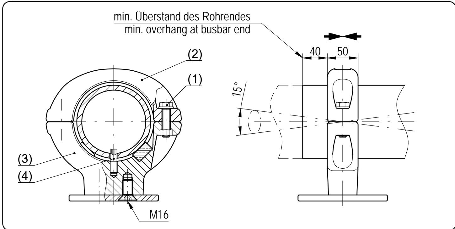
2) Mount tube support together with base plate onto the supporting insulator.
