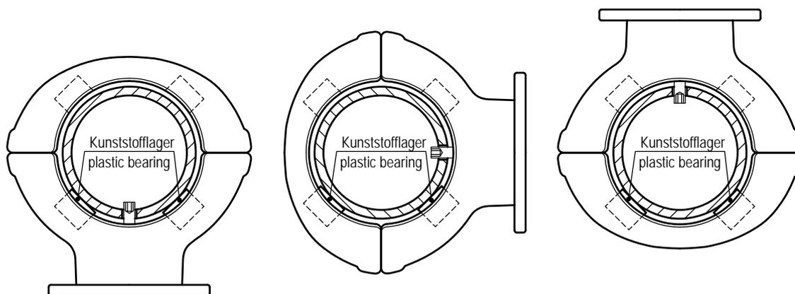
1) For mounting positions sideways and suspensory change the plastic bearing elements. For this purpose prise out the accordant element with a screwdriver and drive it in at the right position with a hammer without damaging the tube support.
